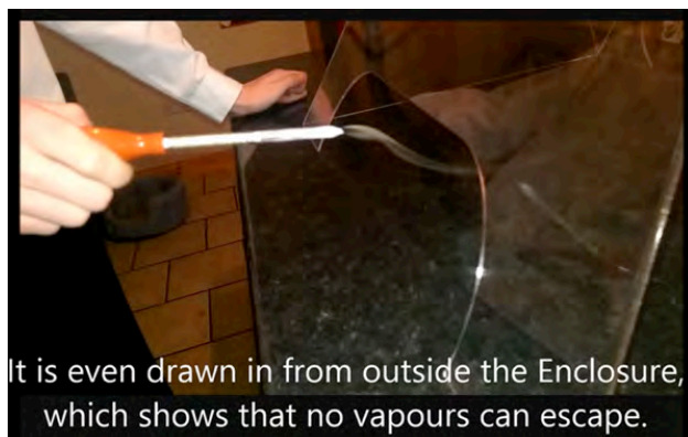
Fig. 3 Extract from demo video: Airflow when extraction is switched on
